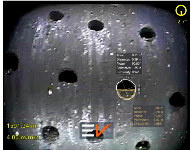
Figure 2: Dimensioned Base Holes Image
