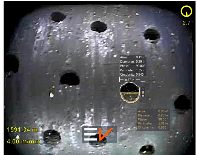
Figure 2: Dimensioned Base Holes Image
