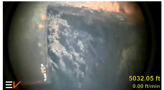
Figure 3: Sideview footage of deformed cut lip guide
