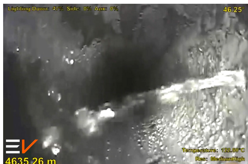
Figure 1: Pin-pointing water entry from a perforation
