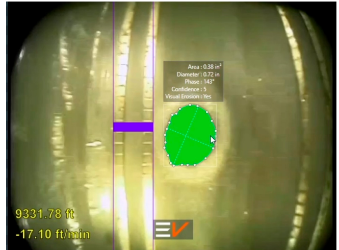
Figure 2: Dimensioned perforation with eroded area calculations
