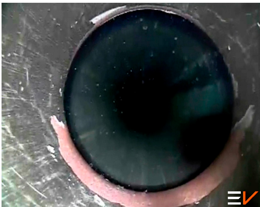
Figure 1: Downview image confirming successful 7 inch casing cut
