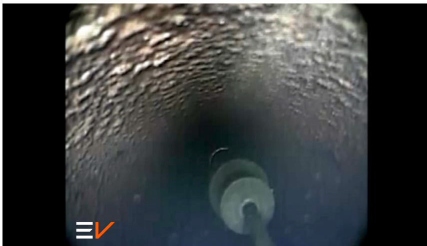
Figure 1: Downview image of stuck tool at 1800m
