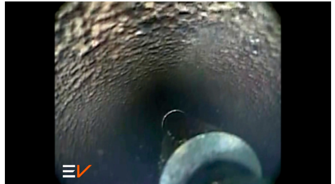
Figure 2: Stuck tool located on lowside of the well
